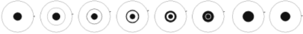
Fig. 1. Distribution of dead zones in the viscosimeter cross-section over the first half-period of the fifth vibration. Mark on the external circle denotes the deviation from the equilibrium position.
